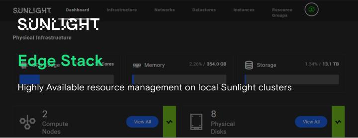
The Sunlight Edge Stack, a component of Sunlight HyperConverged Edge (HCE), provides a graphical management interface onto any Sunlight cluster – including resource-limited Edge clusters. It provides Highly Available local resource management on a single pane of glass. Manage all of your VMs on a local Sunlight cluster, with fine-grained control of your resources.
